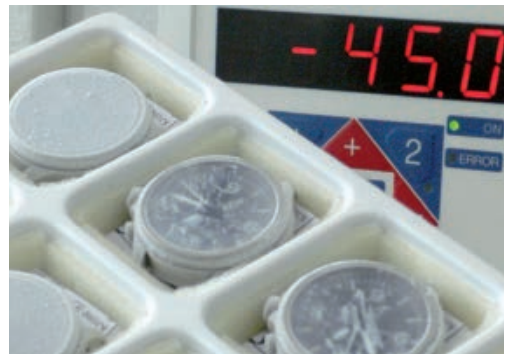
Each and every watch is tested in a temperature chamber at -45^{\circ}\text{C} to +80^{\circ}\text{C} .
