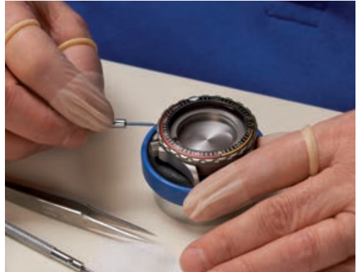
During final assembly, the individual components are pieced together to form complete cases, as shown here by the EZM 7 mission timer for the fire service.
