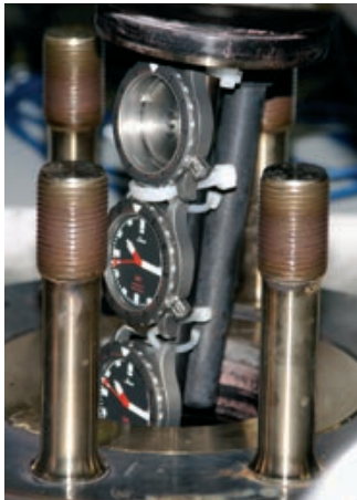
Two U1 models as well as a case are lowered into the pressure chamber.
