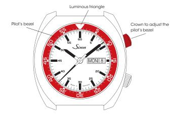
The pilot's bezel can be moved manually in both directions and is adjusted with the crown in the 2 o'clock position. The triangle glows in the dark.
