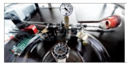
Differential pressure test: The EZM 10 must withstand alternating ambient pressure levels.
