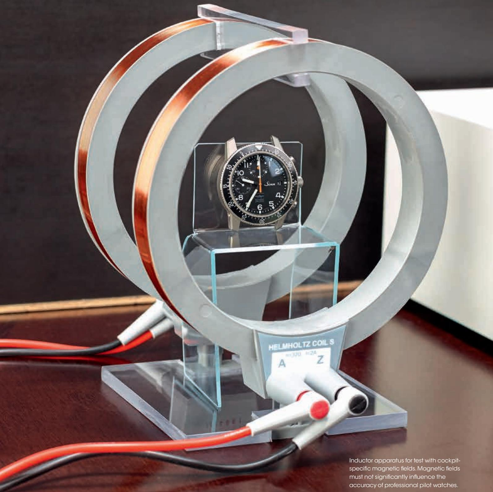
Inductor apparatus for test with cockpit-specific magnetic fields. Magnetic fields must not significantly influence the accuracy of professional pilot watches.
