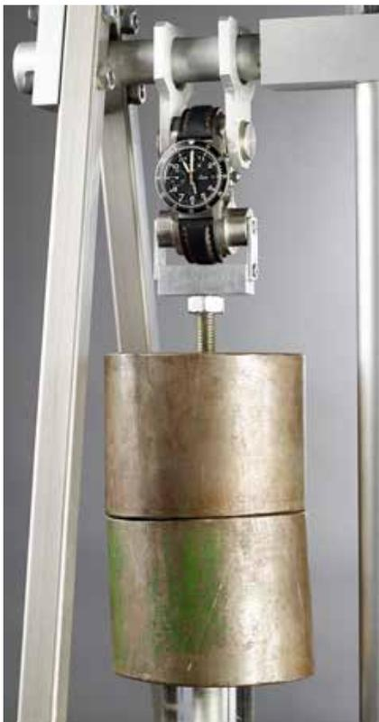
Test facility for testing the safe fastening of the strap system.
