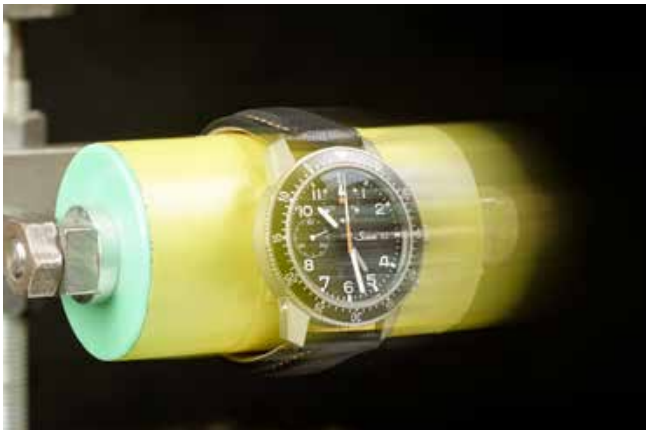
103 Ti UTC IFR in a centrifuge to test G-force load. It is being tested with a load of six Gs.
