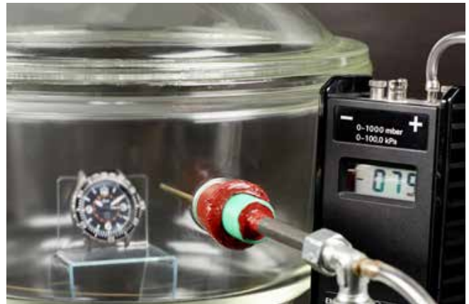
Differential pressure testing in a vacuum desiccator: a DIN 8330-certified pilot watch like the 857 UTC VFR has to be able to withstand several-thousandfold alternating pressure loads.
