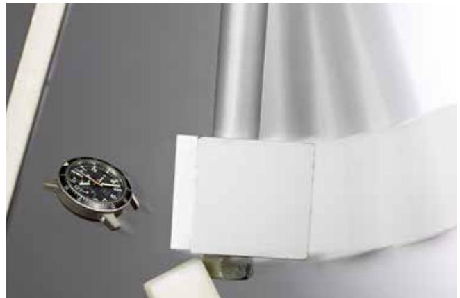
Test facility for testing shock and impact resistance. The 103 Ti IFR is being tested here.
