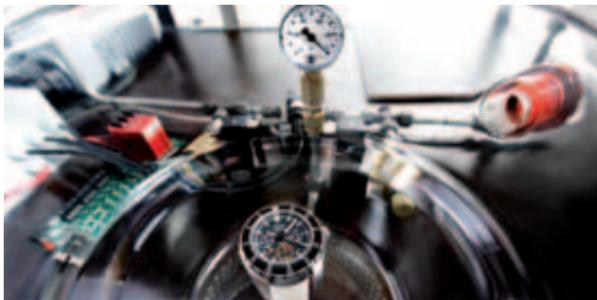
Differential pressure test: The EZM 10 must withstand alternating ambient pressure levels.
