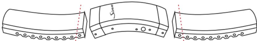
3. Remove the first metal pin and replace it with the spring bar. Then reattach the clasp to the band.
