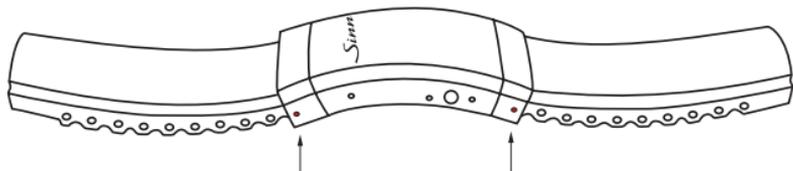
2. Using a knife or scissors, cut the silicone band in the middle between two metal pins. You should shorten the band symmetrically and little by little, starting from the clasp, until you have reached the desired length. Test the length from time to time before proceeding. Shortening both ends by the length of one metal pin results in a total difference of 10 mm in the length of the strap; shortening one end reduces the length by 5 mm.
