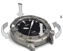
2. Hold down the bezel and turn it anti-clockwise to the desired set time. Once you release the bezel, the rotation protection is reapplied and the bezel is once again prevented from being accidentally adjusted.
