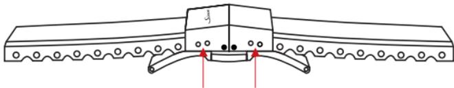
2. Using a knife or scissors, cut the silicone band in the middle between two metal pins. You should shorten the band symmetrically and little by little, starting from the clasp, until you have reached the desired length. Test the length from time to time before proceeding. Shortening both ends by the length of one metal pin results in a total difference of 10 mm in the length of the strap; shortening one end reduces the length by 5 mm.
